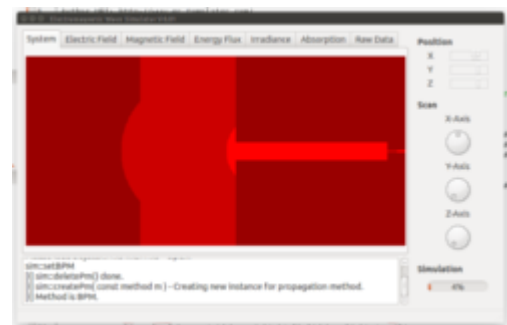
3D-distribution of complex refractive index for definition of the system to simulate.
