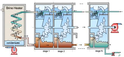
Fig. 1 Schematic representation of a MSF desalination plant
