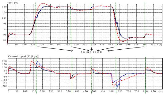
Fig. 9 Simulation results without and with bumpless switching
